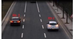
**Figure 3.** An example image showing the detected vehicles and their assigned id's. The vehicles are assigned id 1 and id 2.
