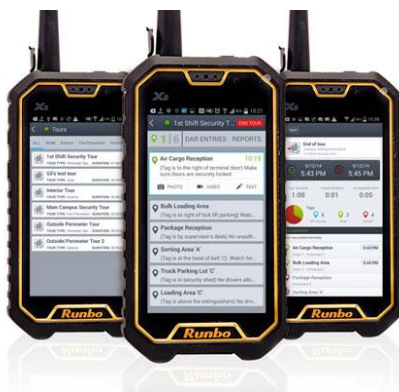
Figure 3. A special device to scan RFID and NFC signals [3].
