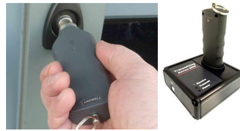
Figure 4. A special device to scan signals from RFID and key [4].
